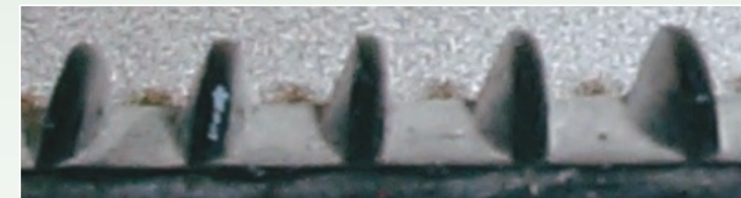
The Sunnybrook rub bars are deeper than the original bars, which helps reduce load spikes on the concave.
