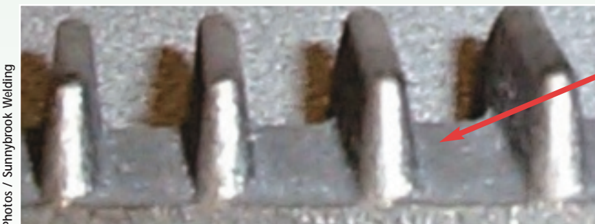
The Sunnybrook rub bars are deeper than the original bars, which helps reduce load spikes on the concave.
