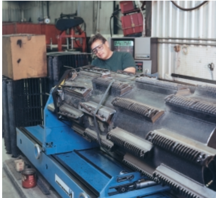
Cylinders are carefully balanced at the shop, and farmers say they keep that balance in heavy harvest conditions.
