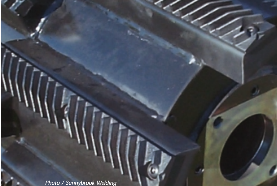
Large Browning hubs on the end plates support the cylinder.
