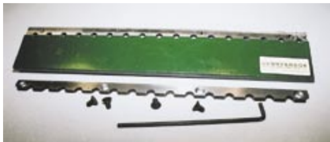
The concave stays in the combine and a simple Allan key allows replacement of a damaged wear edge.
