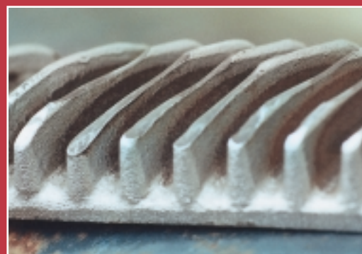
Chrome coating shows wear and surface chipping.
