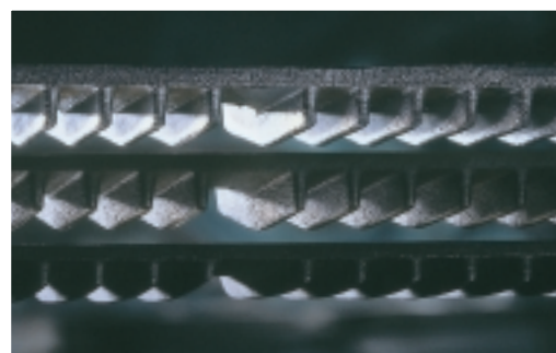
Top: Chrome plated rub-bar. Middle: Boron treated rub-bar. Bottom: Untreated rub-bar.
