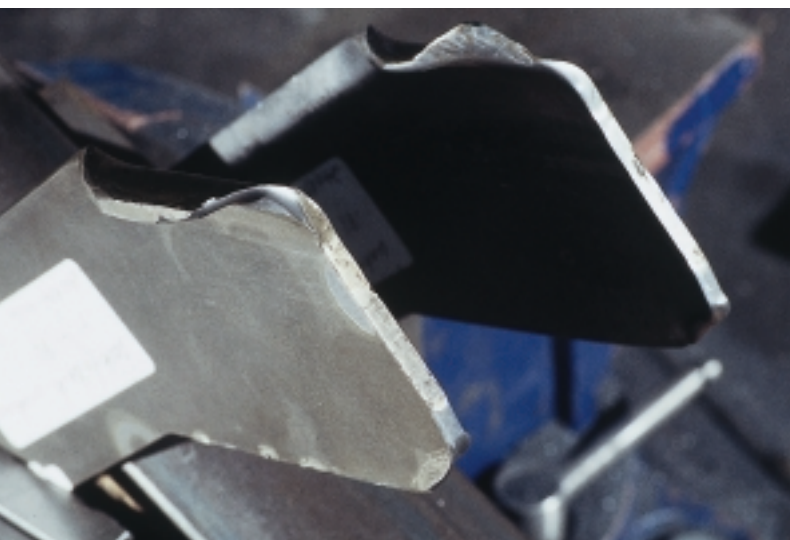
Top: Untreated worn face, thinned to bent over, with some rock dents. Bottom: Boron treated, slight wear and some denting from rocks.
