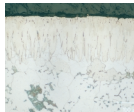
This photo of boronized metal, magnified 100 times, shows a 0.006” layer plus sawtooth penetration deeper into the metal.
