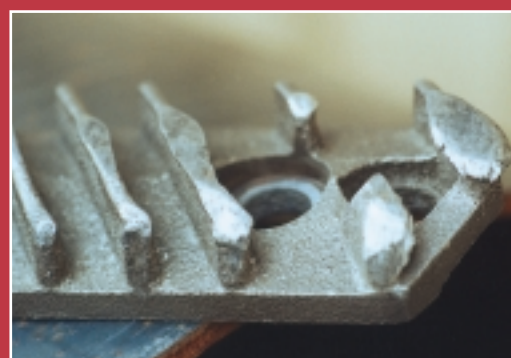
Boron-treated steel rub-bar after a rock impact.
